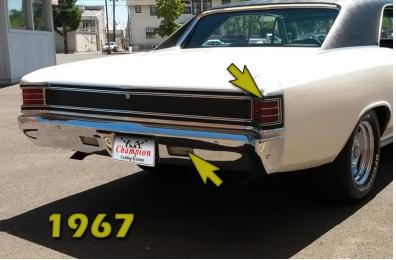
At the rear of the 1966 Chevelle, the reverse lamp is part of the tail lamp, which sits inside of the quarter panel. For 1967, the reverse lamp moves to the bumper, and the tail lamp wraps around the quarter panel.
