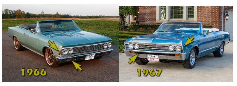
From the front, the 1966 Chevelle grille is angled back from top to bottom, giving the headlamps a protruded look, and for 1967 the lamps a little inboard and the fender line is near vertical. The bumper for 1966 has two slots, split by the license plate area, and for 1967 the slot goes all the way across the bumper and captures the turn signal lamps within.
