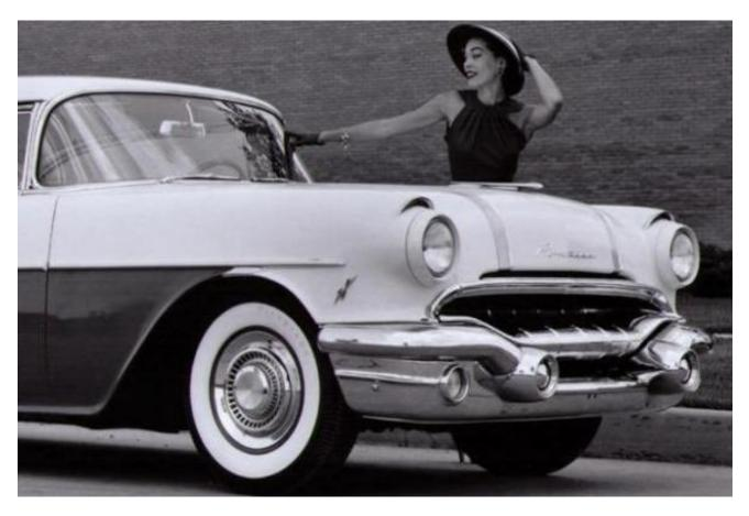
With its minor facelift, the '56 is similar to the previous year, but note that the front bumpers have a 30-degree crook toward the center, while the '55 bumpers are straight. That's one easy tell to distinguish the two model years. Also, all the metalwork in the grille opening is bright rather than painted.
